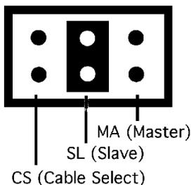
tion jumper. It is a set of six pins with a plastic jumper on two of them. There are three jumper positions: CS (Cable Select), SL (Slave), and MA (Master). The CD-ROM drive leaves the factory set as a slave. Have it set as slave for this configuration.
