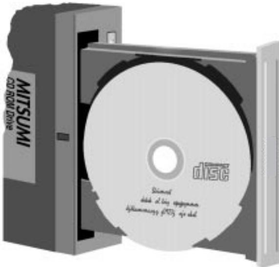
with 4 notches may be installed with the eject button at either the top or the bottom. Before installing or removing the CD-ROM drive, make sure that there is no disc in the drive and that the disc tray is closed.
